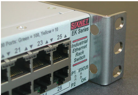
In the image above, the brackets are mounted so the front of the switch is setback 1/2 inch.
